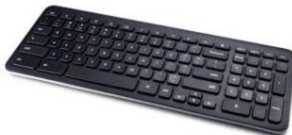
A computer keyboard is one of the primary input devices used with a computer that looks similar to those found on electric typewriters, but with some additional keys. The modern keyboard is based on the
