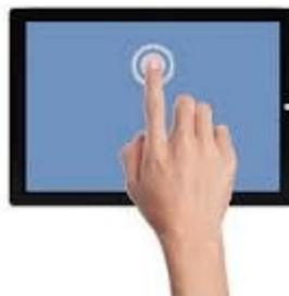
A touchscreen is a monitor or other flat surface with a sensitive panel directly on the screen that registers the touch of a finger as an input. Instead of being touch-sensitive, some touchscreens use beams across the screen to create a grid that senses the presence of a finger.
