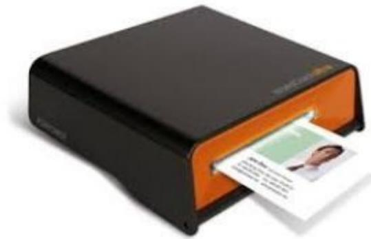
a business card reader allows a user to scan business cards into their computer for digital storage. Computer scanners are capable of scanning and converting text documents to typed text by use of Optical Character Recognition (OCR) software. Business card readers work on a similar principle, reading the text on the business card and converting to typed text on the computer.
