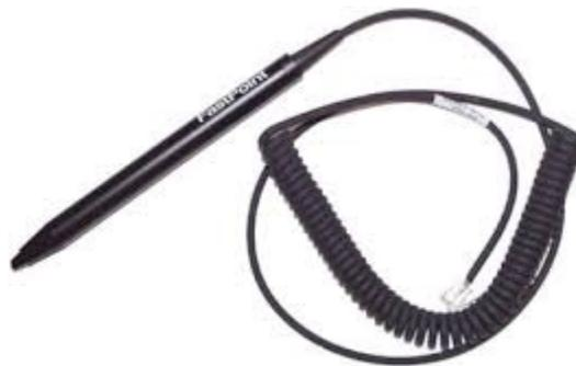
A light pen is a computer input device in the form of a light-sensitive wand used in conjunction with a computer's CRT display. It allows the user to point to displayed objects or draw on the screen in a similar way to a touchscreen but with greater positional accuracy. A light pen can work with any CRT-based display and other display technologies, but its ability to be used with LCDs was unclear (though Toshiba and Hitachi displayed a similar idea at the "Display 2006" show in Japan).
