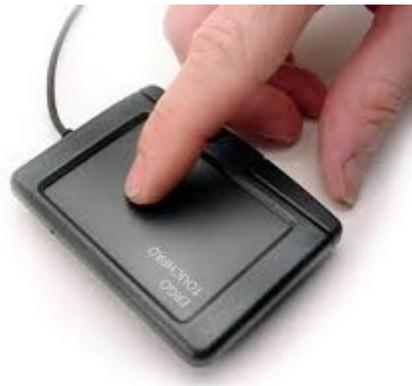
a touchpad is an input device on laptops and some keyboards to move a cursor with your finger. It can be used in place of an external mouse.
