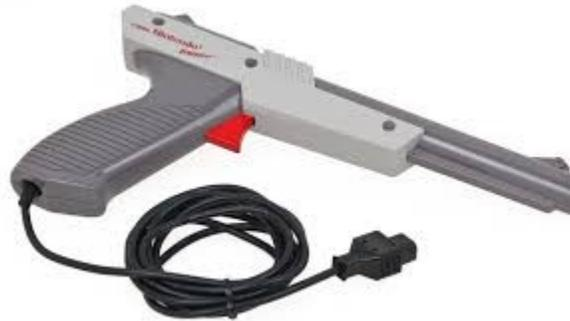
A light gun is a pointing input device that detects light using a photodiode in the gun barrel. When the player of the game pulls the trigger on the gun, the screen is blanked out for a fraction of a second, which allows the photodiode to determine where the gun is pointed. Light guns were most widely used with early console gaming systems such as the NES Zapper light gun, as shown in the picture
