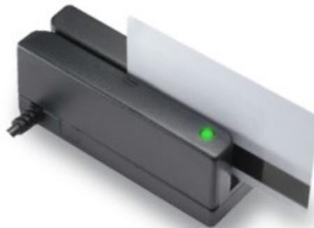
A magnetic card reader is a device that can retrieve stored information from a magnetic card either by holding the card next to the device or swiping the card through a slot in the device. The picture is an example of a magnetic card reader and a good example of the type of card reader you would see at most retail stores.
