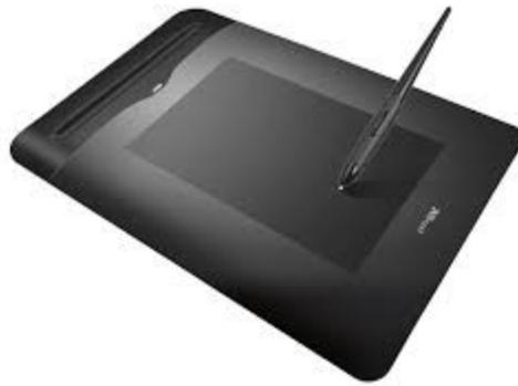
a graphics tablet is a hardware input device that enables an artist to draw or sketch digitally using a pen or stylus. They are helpful because they provide a more natural and precise feel than a standard computer mouse. The picture to the right shows an example of a Pen Graphics Tablet from Wacom.
