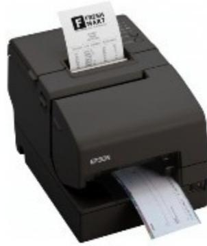
Magnetic Ink Character Recognition Code (MICR Code) is a character-recognition technology used mainly by the banking industry to ease the processing and clearance of cheques and other documents. The MICR encoding, called the MICR line, is at the bottom of cheques and other vouchers and typically includes the document-type indicator, bank code, bank account number, cheque number, cheque amount, and a control indicator.
