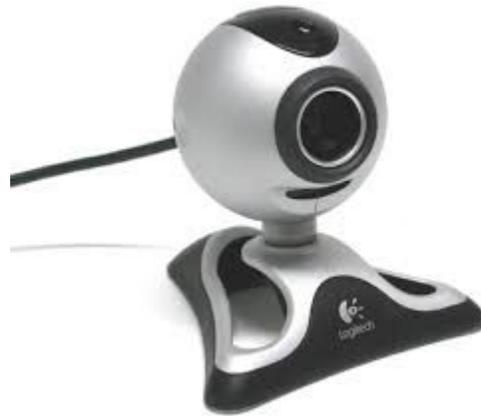
A webcam is a hardware camera connected to a computer that allows anyone connected to the Internet to view either still pictures or motion video of a user or other object.
