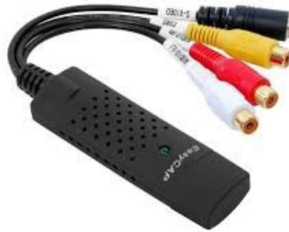
The video capture device is then capable of taking that video signal and converting it to a stored video format, allowing you to store, modify, and show video on a computer.
