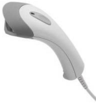
A barcode reader (BCR) or scanner, also known as a point of sale (POS) scanner is a hardware device capable of reading a barcode. It can also print out the details of the product or log information about that product into a database. A perfect example of a barcode reader is a super market barcode scanner that reads and logs the price of a product. In the picture is an example of a Barcode reader from HP.
