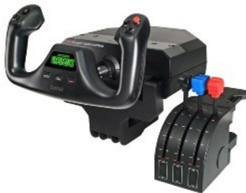
A yoke is a hardware input device used with computer games, such as flight simulation games, that allow a player to fly up or down, or back or forth by pulling or pushing the device.
