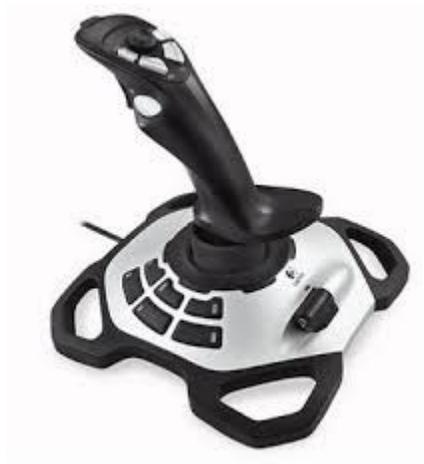
A joystick is an input device that allows the user to control a character or machine in a computer program, such as a plane in a flight simulator. They look similar to the control device you would find on an arcade game, but nearly always include extra buttons for additional functionality. The picture shows the Logitech Freedom 2.4, an example of a joystick.
